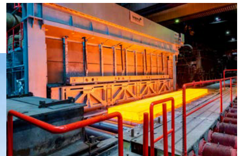
Low energy, top quality: the starting materials often used in the automotive industry are preheated in a process gentle to surfaces in the new walking beam furnace in Duisburg.
